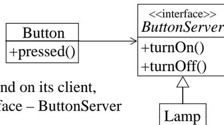
An interface does not depend on its client, thus, the name of the interface – ButtonServer
