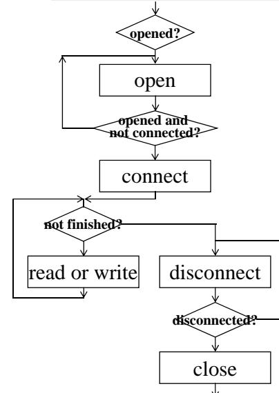
This is the control flow for the TYPICAL / CORRECT usage of this NetCommStream object.
