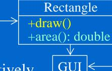
2 area() and draw() are two unrelated responsibilities If Graphical Application causes draw() to change or GUI changes somehow, these changes force us to rebuild, retest, and redeploy the Computational Geometry Application.
